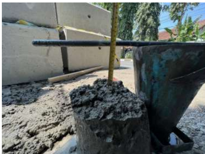
Gambar 4.19 Slump Test Redymix (Sumber : CV. Progresif Quality Planning, 2023)
