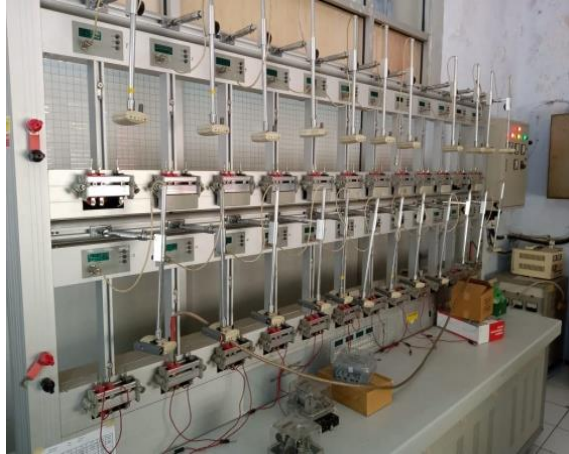
Gambar 2.25 Test Bench kWh Meter Standar Hsiangcheng
