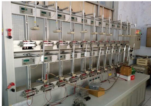
Gambar 2.14 Test Bench kWh Meter
